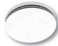
The ComfoValve Luna S125 supply valve is equipped with a detachable design cover. Therefore this valve can stay in the wall or ceiling during cleaning.
